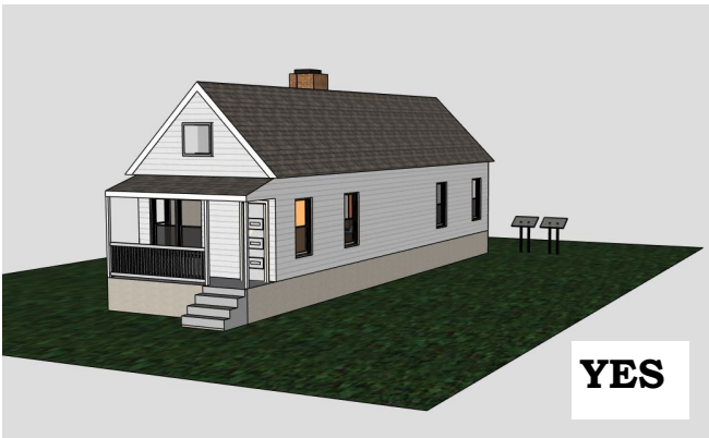
Solar panels should not be added on prominent roof locations but instead be placed towards rear rooflines or free-standing in yards.
